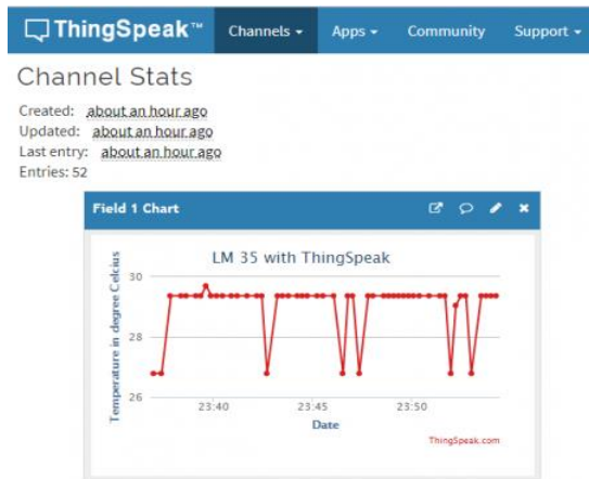
Figure 8: IoT Temperature Data Logger Using ESP8266 and LM35 – ThingSpeak Graph
