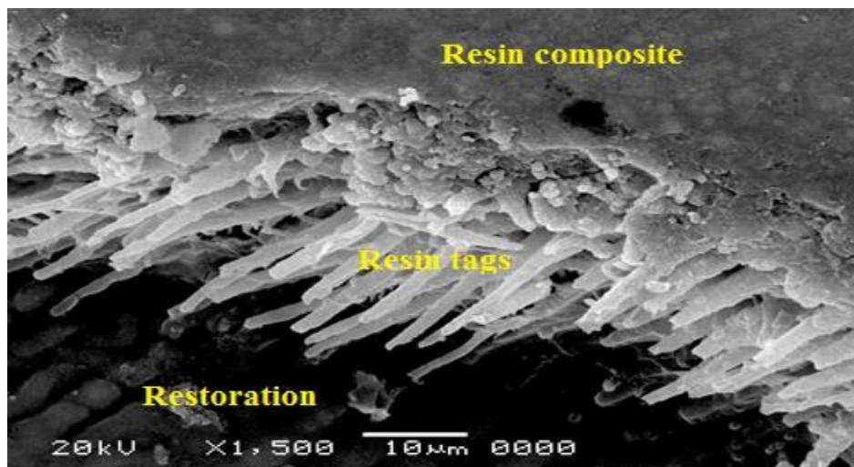
**Figure (5):** Scanning electron photomicrograph for the resin dentin interface (at 1500X) of Silorane at 6 months storage showing gap at the interface.
